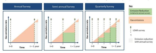
Figure 11: Schematic overview of emission reductions within a year depending on the frequency of the surveys
