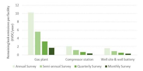
Figure 13: Average remaining leak emissions per facility depending on the survey frequency<sup>22</sup>
