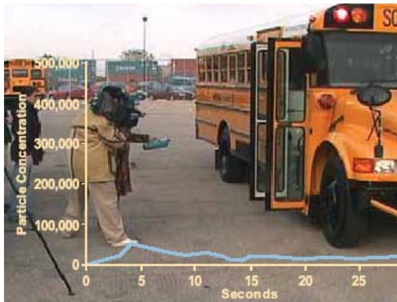
The bus retrofit with a particulate matter filter leaves no particulate matter plume behind as it pulls away from a bus stop or school.
