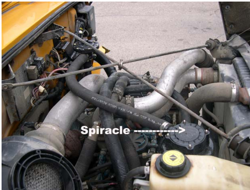
A crankcase ventilation filtration system, the Donaldson Spiracle (black canisters connected by black hose on top of engine) reroutes crankcase emissions through the exhaust system and emissions controls.
