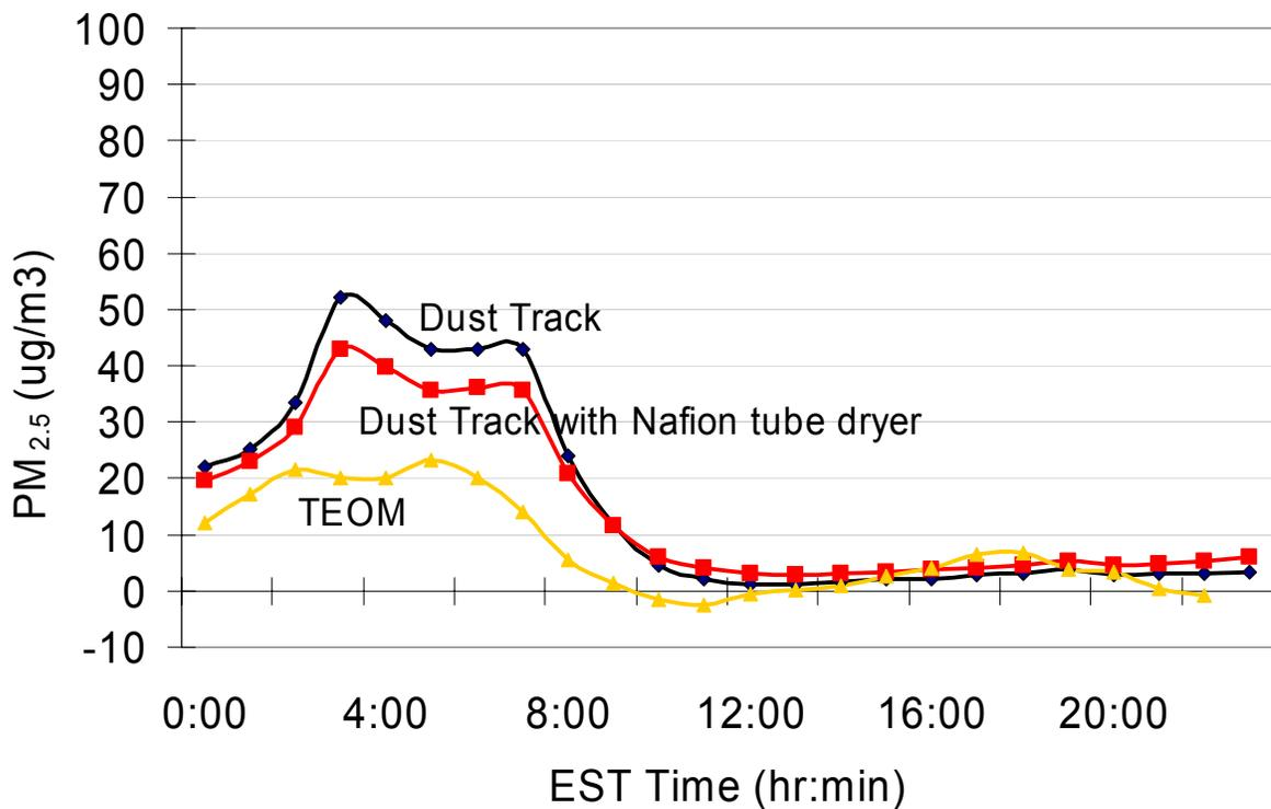
*Figure 6: Comparison of Dust Trak to TEOM in Gorham NH. Note site is rural and dominated by sulfates. Suggests Dust Trak with Nafion tube dryer overpredicts PM<sub>2.5</sub> levels roughly by a factor of 2 when the Nafion Tube dryer is used.*
