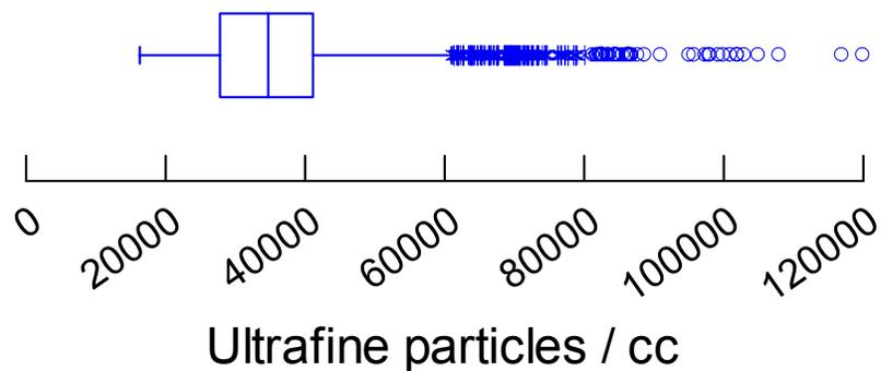
**Figure 19: Distribution of in-cabin ultrafine particulate matter levels in the bus equipped with a DOC. Compared to Figure 13, the ultrafine PM remains elevated at levels similar to the conventional bus, but with the DPF-ULSD combination, cabin levels are cut to ambient. This suggests that the DOC has limited usefulness as a device to improve in-cabin ultrafine PM.**
