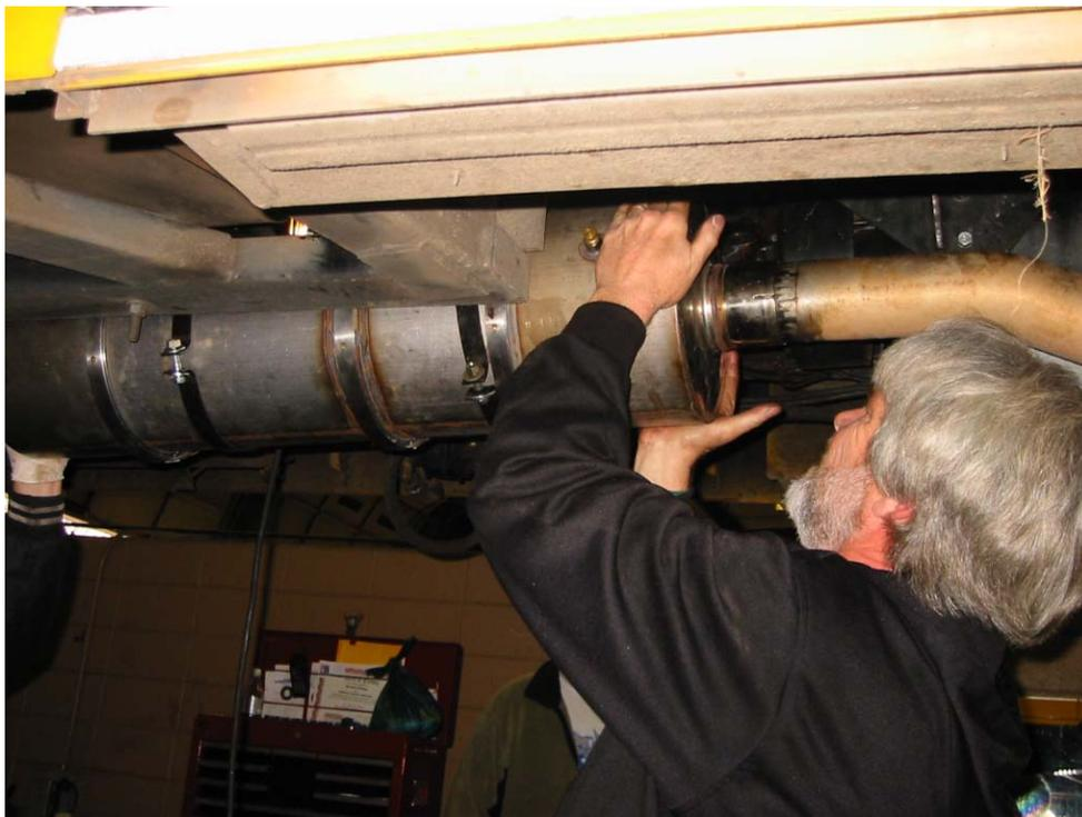
***Figure 3: Installation of diesel particulate filter on DeKalb bus prior to testing.***
