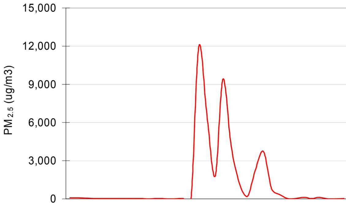
**Figure 25:** Raw PM<sub>2.5</sub> concentrations approximately one meter from tubing connected to the road draft tube on the retrofit bus. These extreme PM<sub>2.5</sub> levels (exceeding 10,000 ug/m<sup>3</sup>) explain why this source –which vents very near the front door of the bus--so strongly impacts in-cabin air quality.
