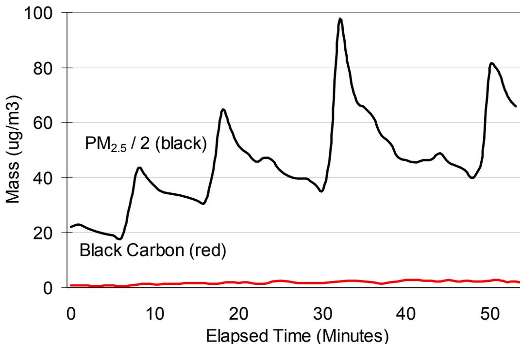
**Figure 36:** A comparison of PM<sub>2.5</sub> (divided by 2.0 to account for Dust Trak overestimate of PM<sub>2.5</sub>) suggests that black carbon accounts for a very small fraction of in-cabin PM<sub>2.5</sub> mass in conventional diesel school buses. Chicago data.
