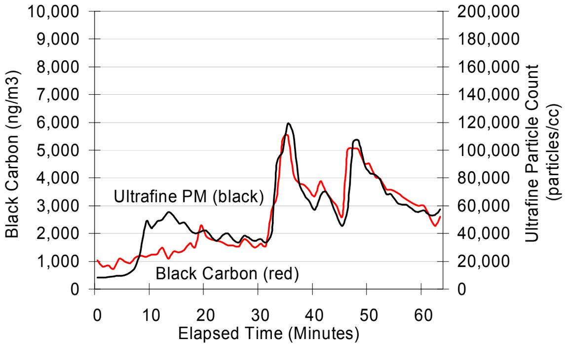
**Figure 37:** Conventional bus with ULSD fuel showed persistent BC and Ultrafine PM in the bus cabin.
