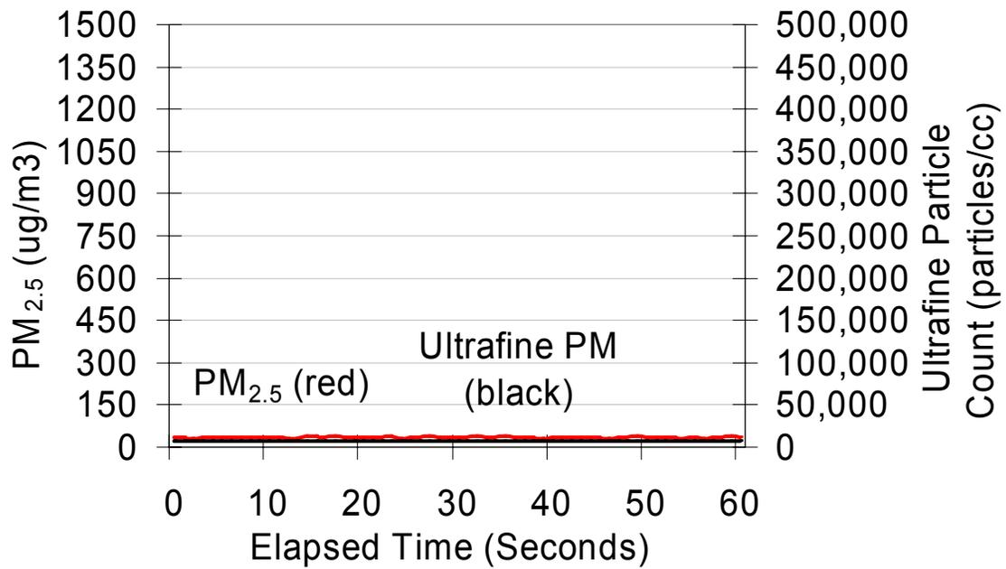
**Figure 49:** Simulation of drop-off scenario on retrofit bus demonstrates elimination of curbside pollution from the bus. DPF-ULSD-Spiracle retrofit.
