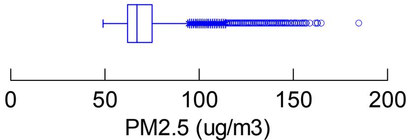
***Figure 23: Fine particulate matter (PM<sub>2.5</sub>) in DPF-ULSD retrofit bus remain high following retrofit. PM<sub>2.5</sub> was found to be a result of direct engine emissions rather than tailpipe emissions.***
