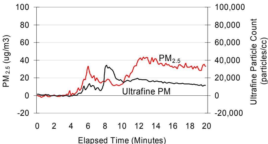
**Figure 42: Idle test of DOC-equipped bus. Ambient concentrations have been subtracted. (Ann Arbor data.)**
