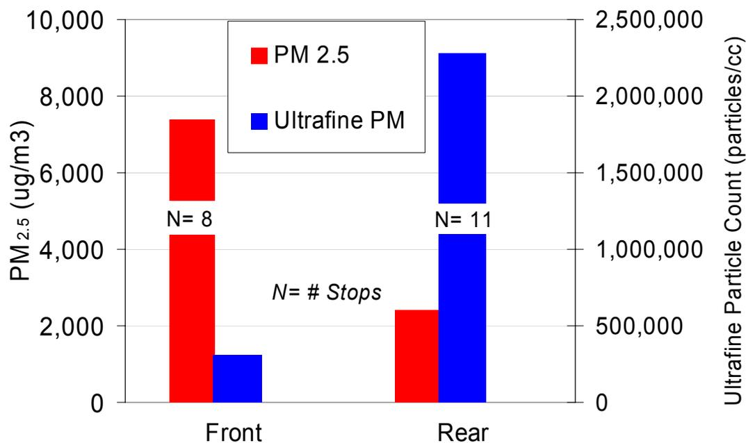
**Figure 15:** Graph shows relationship between wind direction and build-up (cumulative peaks) of ultrafine PM and PM<sub>2.5</sub> on the conventional bus with conventional fuel. PM<sub>2.5</sub> is highest when wind blows from the front of the bus (crankcase emissions) and
