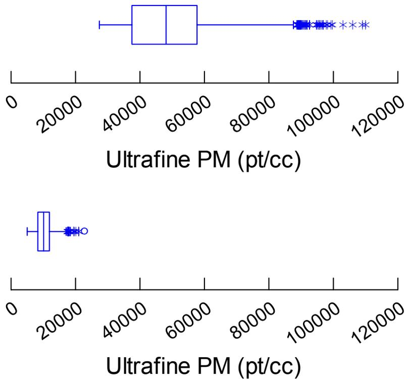
**Figure 17:** *Box plots display the range of ultrafine particulate matter concentrations measured in a conventional school bus (top plot) and later equipped with DPF-ULSD in Atlanta (lower plot). Note there is little or no overlap between ultrafine particle ranges in conventional buses and buses equipped with DPF – ULSD retrofit. Measured levels on the bus are near ambient levels (17,000 pt/cc that day).*
