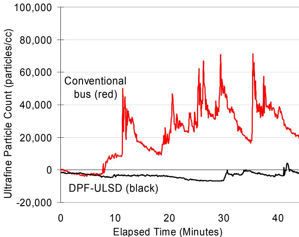
**Figure 18: Comparison of cabin air quality before and after retrofit. Spikes in the conventional bus curve occurred at bus stops when exhaust from the tailpipe entered front door. These spikes were eliminated by the DPF-ULSD retrofit. (Atlanta data). Ambient concentrations have been subtracted from the data resulting in the slightly negative concentration range.**
