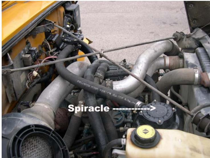
**Figure 31:** Donaldson’s closed crankcase filtration device, the Spiracle was installed in combination with a conventional bus, a DPF-ULSD retrofit bus, and a bus with a DOC. The Spiracle eliminated the PM<sub>2.5</sub> self-pollution in the cabin of the bus.
