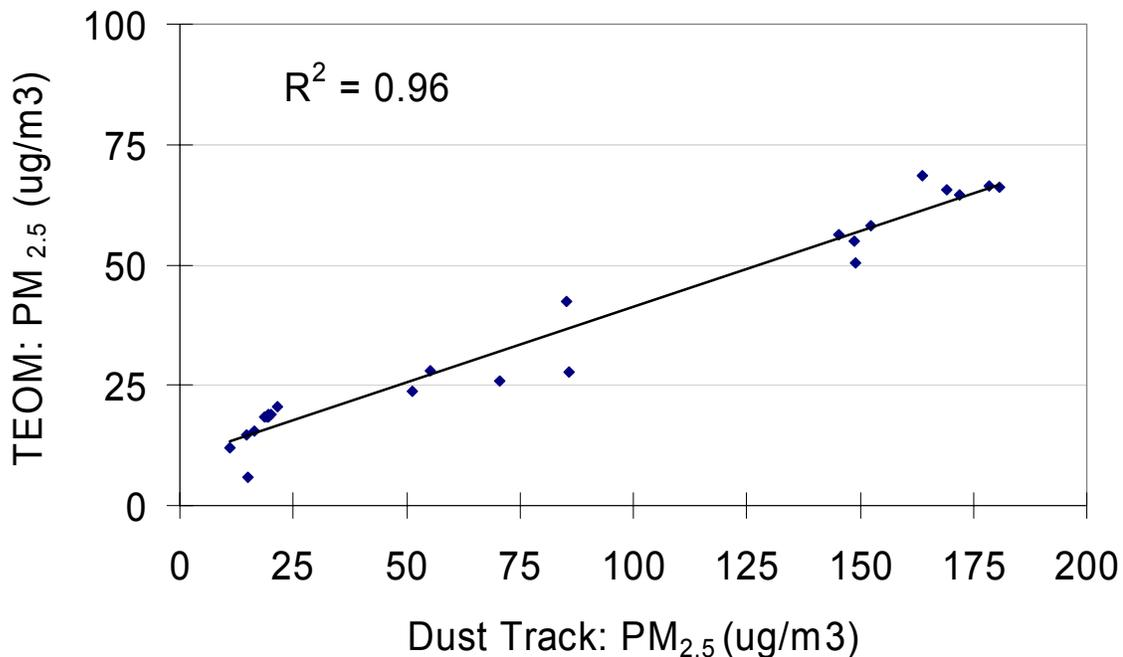
*Figure 7: Linear regression of Dust Trak vs TEOM response on August 30, 2004.*
