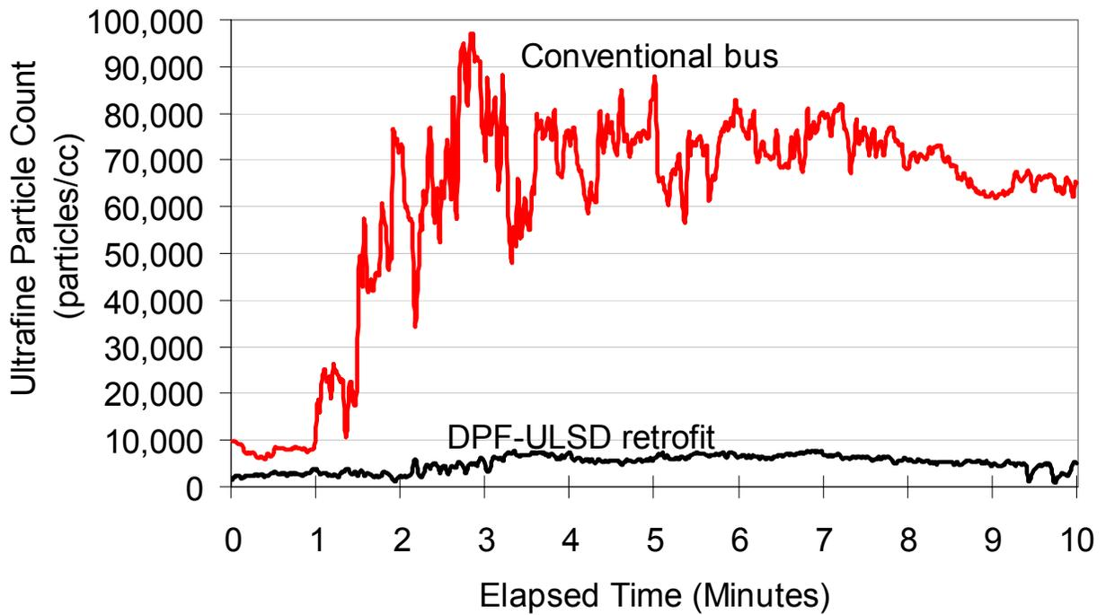
**Figure 45:** In this 15 minute idle test of a Chicago bus, ultrafine particle levels rose rapidly. In contrast a Naperville, IL bus (ULSD-DPF) remained at ambient conditions. Ambient ultrafine concentrations have been subtracted from both curves.
