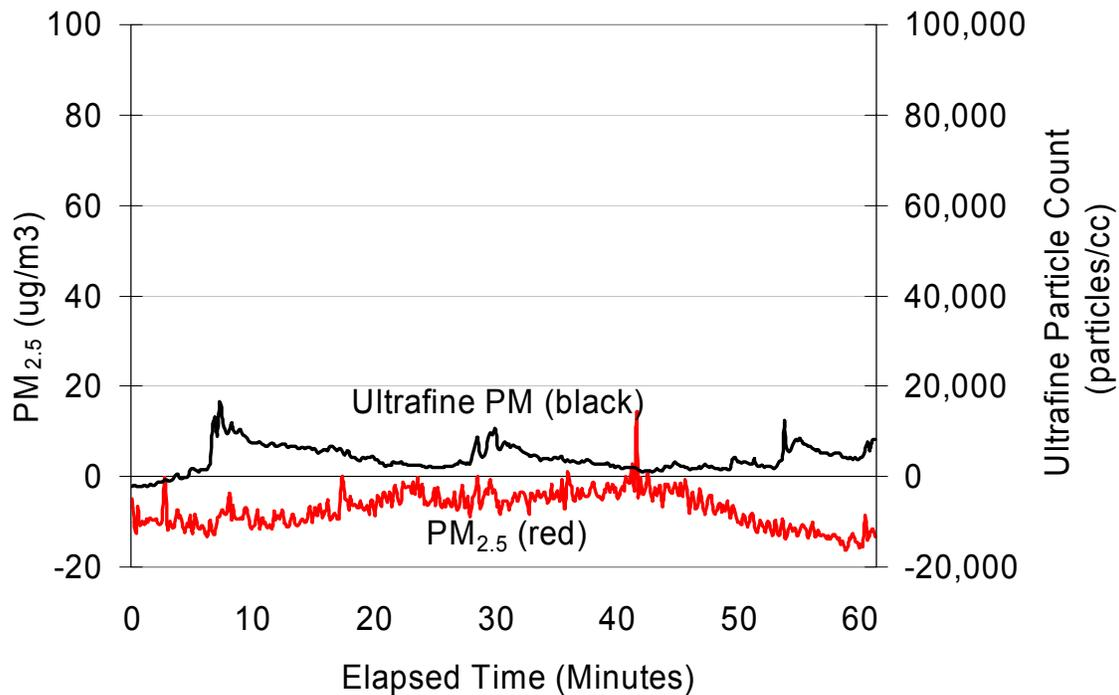
*Figure 33: Net ultrafine particles and  $PM_{2.5}$  concentrations on bus equipped with a DPF-ULSD-Spiracle. The DPF-ULSD-Spiracle combination eliminated all monitored particulate matter self pollution ( $PM_{2.5}$ , ultrafine particles, black carbon and particle-bound PAH.) on the bus. Ambient concentrations have been subtracted.*
