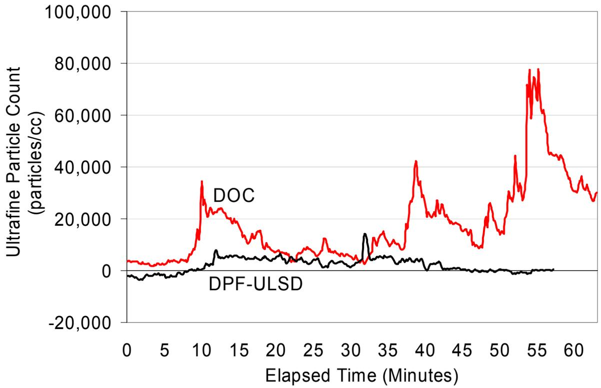
**Figure 20: Net cabin ultrafine pollution, comparing DPF vs DOC in reducing ultrafine particles. Ambient concentration has been subtracted. The DPF remains near ambient the entire bus route.**
