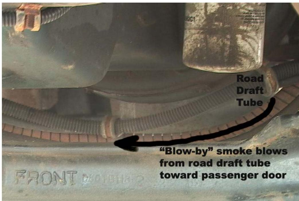
**Figure 28:** Single frame from video from under front end of bus showing diffused smoke emitted by the engine crankcase road draft tube. When wind blew from the driver’s side of the bus toward the open cabin door, a plume of “blow-by” smoke entered into the cabin, dramatically increasing particulate matter levels inside the bus.
