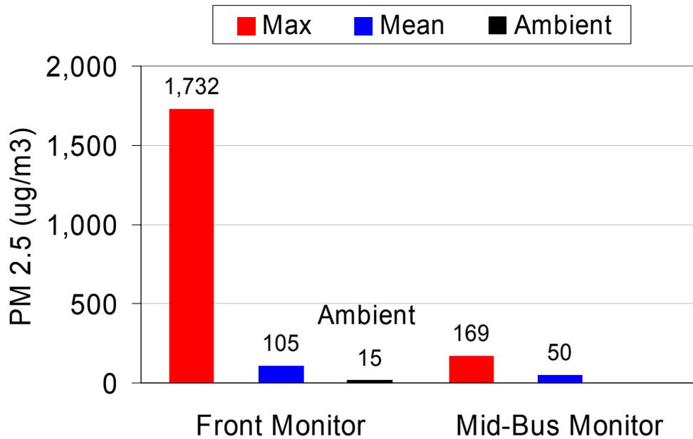
**Figure 9:** Comparison of  $PM_{2.5}$  levels between front and mid bus monitors. In all three cities, crankcase exhaust was documented entering bus through door, thus levels are systematically higher in the front of the bus than mid bus.
