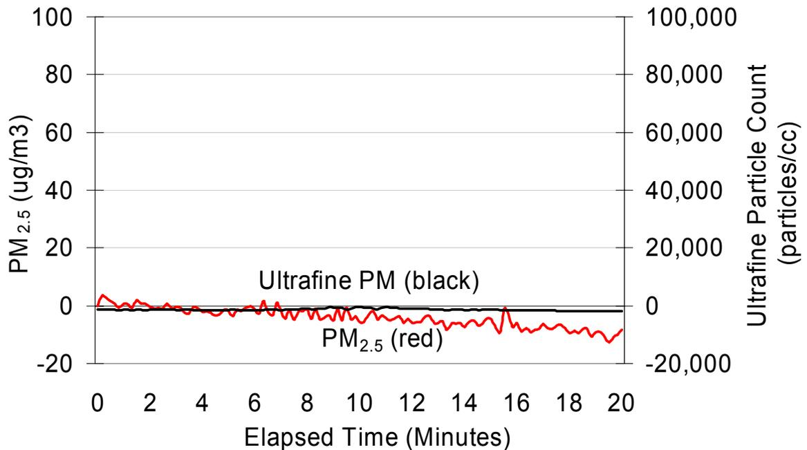
**Figure 46:** Idle test of bus retrofit with DPF-ULSD-Spiracle combination showing elimination of self-pollution. Ambient concentrations have been subtracted.
