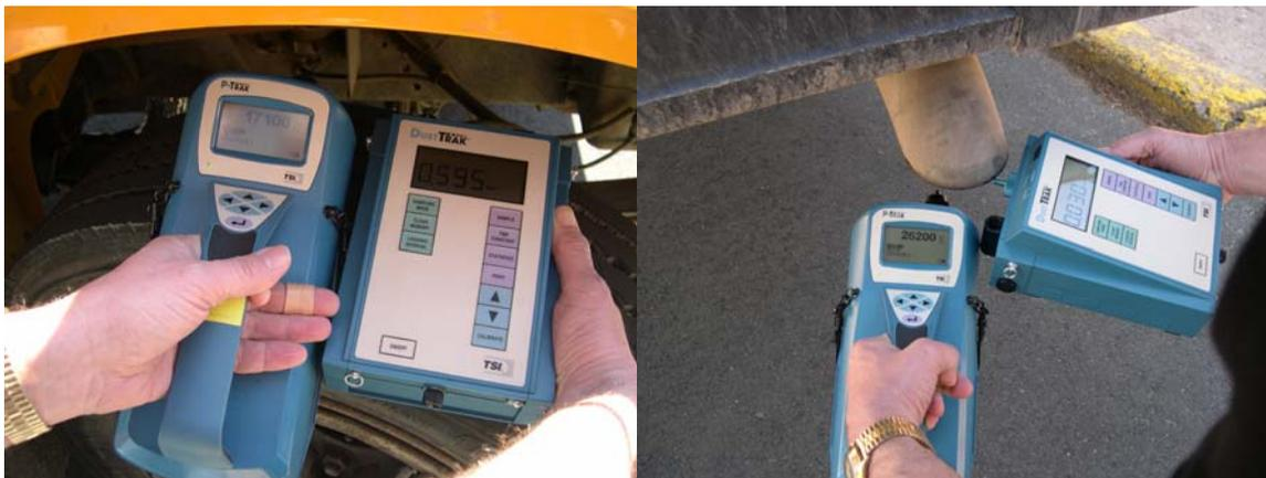
**Figure 26:** In a simple experiment, the Dust Trak (rectangular instrument) responded strongly to PM<sub>2.5</sub> from engine crankcase smoke from the road draft tube (left photo). The PTrak (instrument with handle) responded strongly to tailpipe emissions (right photo).
