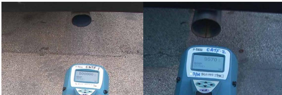
**Figure 16: A simple tailpipe demonstration of the effectiveness of the DPF-ULSD combination in reducing ultrafine PM to ambient conditions . Conventional bus (on left) reads 500,000 ultrafine particles/cc, the upper limit of detection for the PTrak. The retrofit bus (on right) reads 9,570 ultrafine particles/cc—levels that were actually below ambient that day.**
