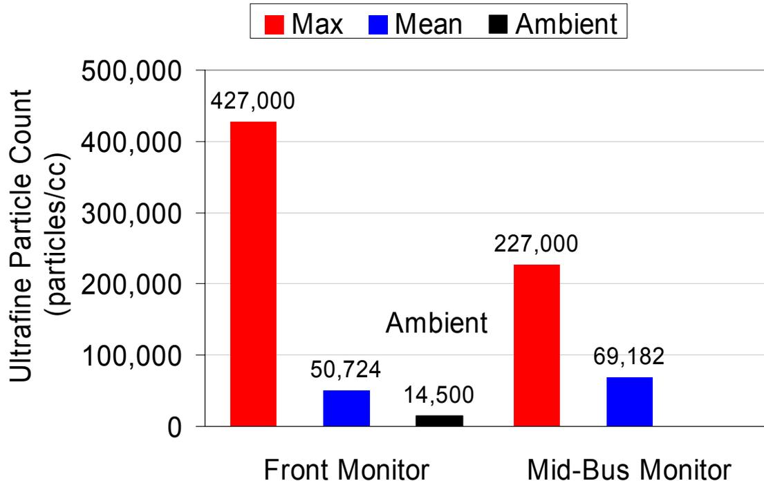
**Figure 8: Comparison of ultrafine PM levels between front and mid bus monitors. In all three cities, tailpipe exhaust was documented entering bus through door, thus levels were typically higher in the front of the bus than mid bus.**
