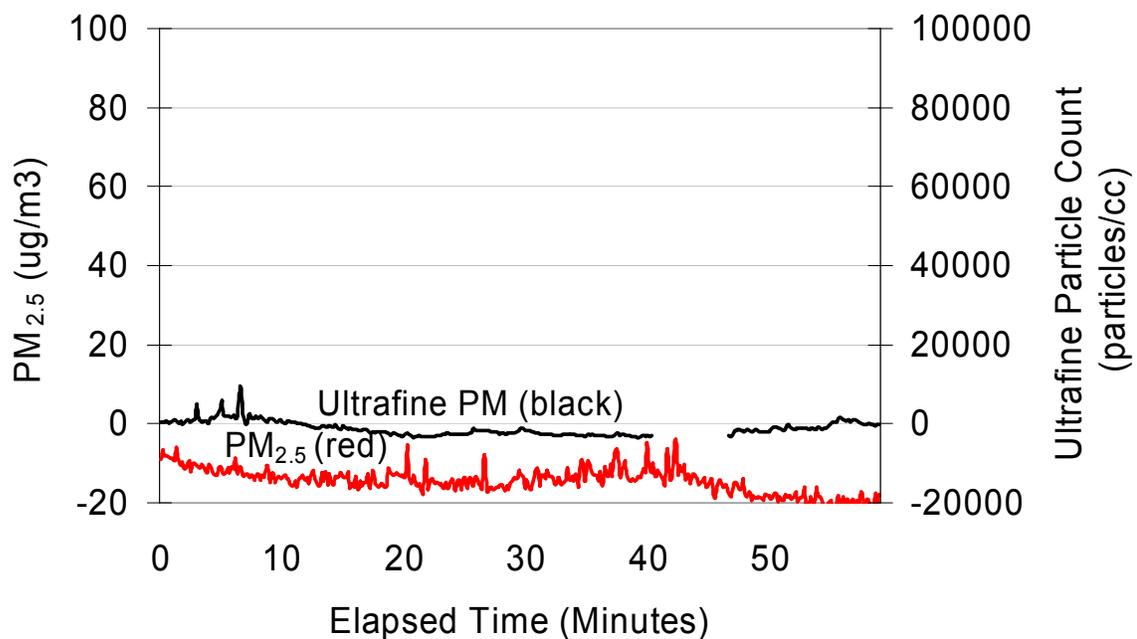
**Figure 2: The DPF-ULSD-Spiracle combination eliminated  $PM_{2.5}$ , ultrafine particles, black carbon, and PAH self pollution from the bus cabin. Ambient concentrations have been subtracted resulting in slightly negative apparent net concentrations. Concentrations below zero should be taken as zero net  $PM_{2.5}$  contribution to the bus.**
