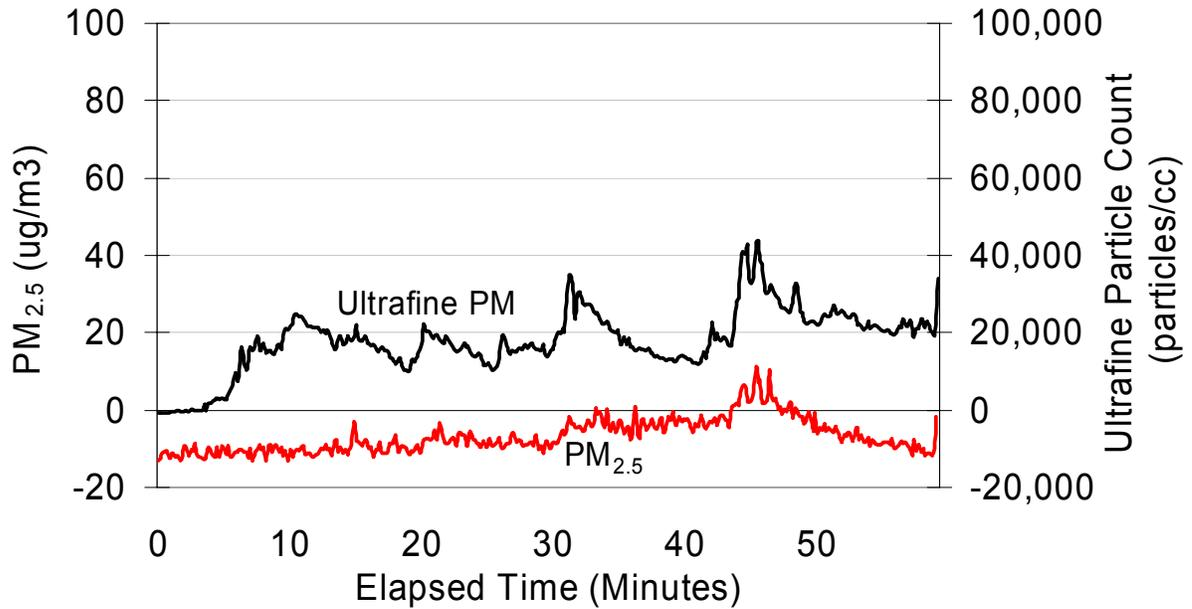
**Figure 58:**  $PM_{2.5}$  and ultrafine particle concentrations on bus retrofit with Spiracle--ULSD shows reduction in cabin  $PM_{2.5}$  approximately to ambient or slightly below. Ultrafine particles remain elevated. Suggests source of cabin  $PM_{2.5}$  is engine crankcase. Ambient concentrations have been subtracted. (Ann Arbor data.)
