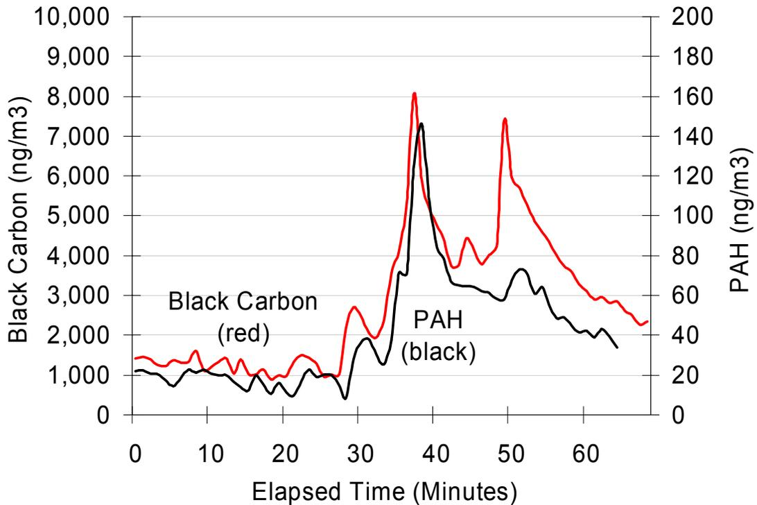
**Figure 38:** PAH and Black Carbon levels remain elevated on the DOC-equipped bus in Ann Arbor, MI.
