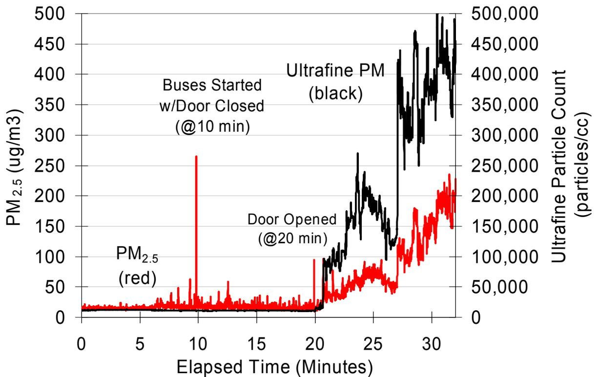
**Figure 44: Results of Ann Arbor bus queue.** Concentrations of both PM<sub>2.5</sub> and ultrafine PM<sub>2.5</sub> remain near ambient with doors initially closed. When doors were opened levels rise very rapidly to levels three times the federal daily PM<sub>2.5</sub> standard and 15 times the federal annual standard in ten minutes. Ultrafine PM levels exceeded 500,000 particles/cc limit of detection.
