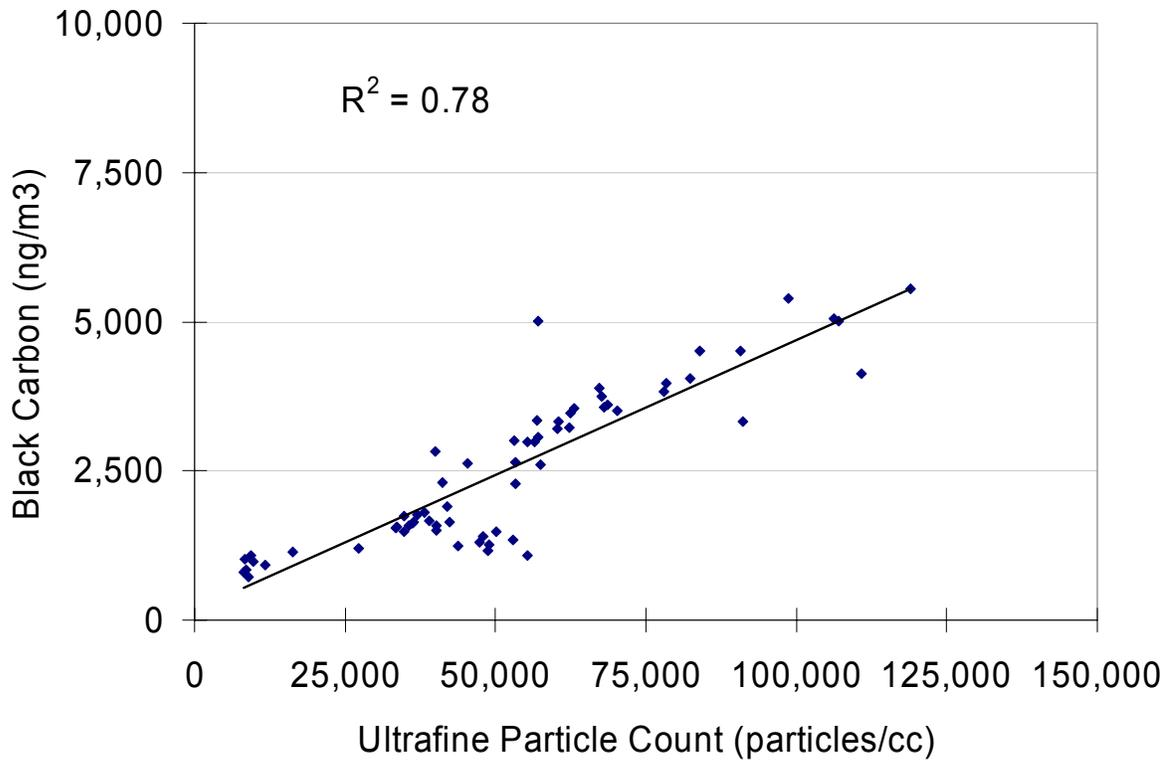
*Figure 54: Linear regression illustrating the close relationship between black carbon and ultrafine particles. Similarly the Pearson’s  $R^2$  in Table 10 suggests a predictable relationship between black carbon and PAH particle emissions (Ann Arbor Conventional bus on ULSD fuel.)*
