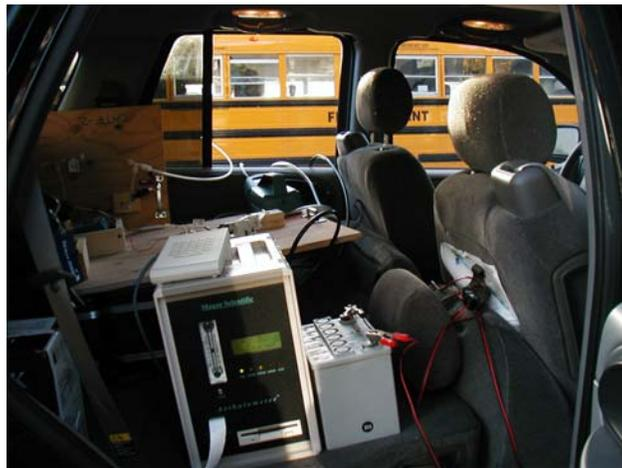
**Figure 50:** Monitoring set up outside elementary school in CT during morning school bus drop off.
