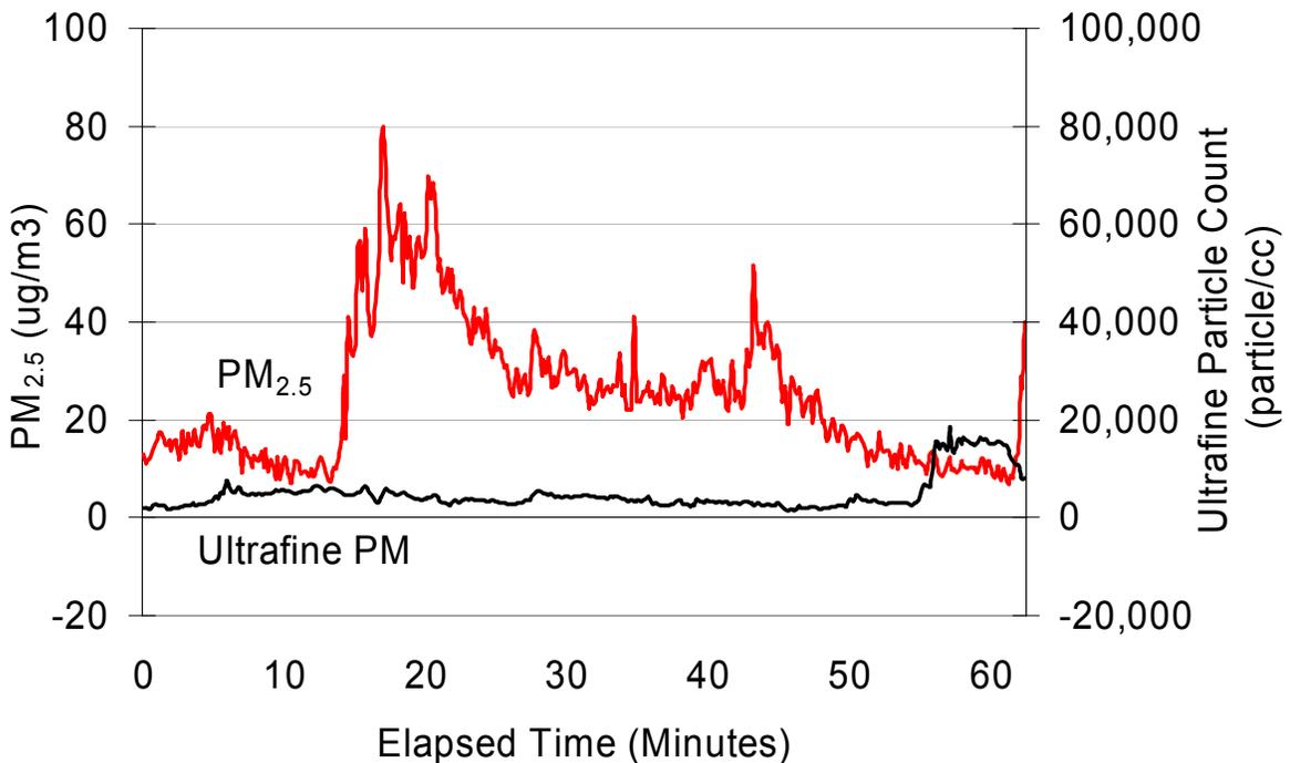
**Figure 57:** *PM<sub>2.5</sub> and ultrafine particle concentrations on bus retrofit with DPF-ULSD shows reduction in cabin ultrafine particles approximately to ambient. PM<sub>2.5</sub> remains elevated, however. Source of cabin PM<sub>2.5</sub> is engine crankcase, not tailpipe,*
