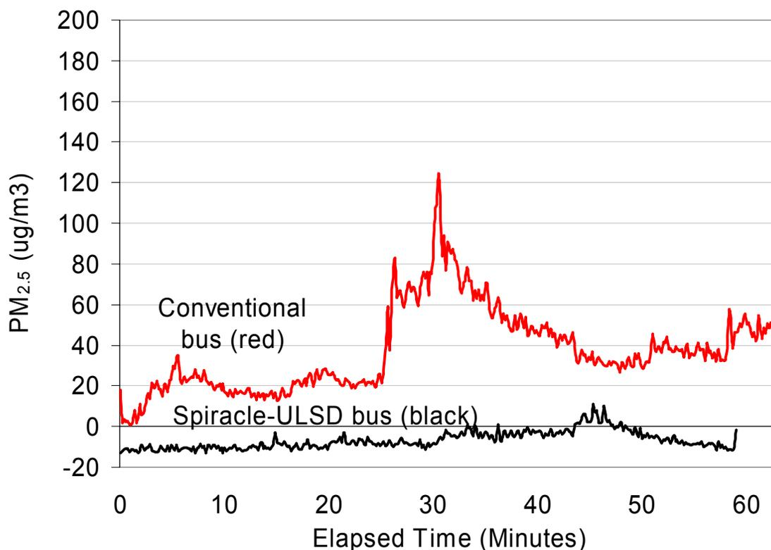
**Figure 35: Comparison of PM<sub>2.5</sub> levels in conventional bus vs Spiracle-retrofit bus. Ambient concentration has been subtracted. (Ann Arbor, MI.)**
