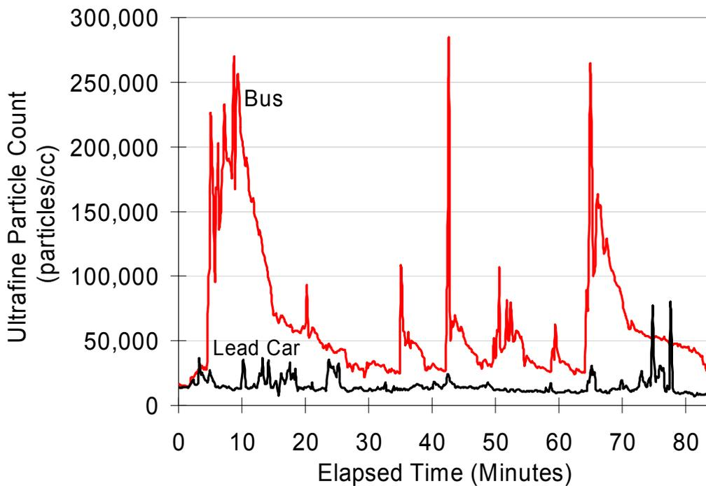
**Figure 12:** *Ultrafine particles in the bus cabin are not from the roadway but instead result from bus self pollution-- as indicated by the low concentrations in the lead car relative to the bus.*
