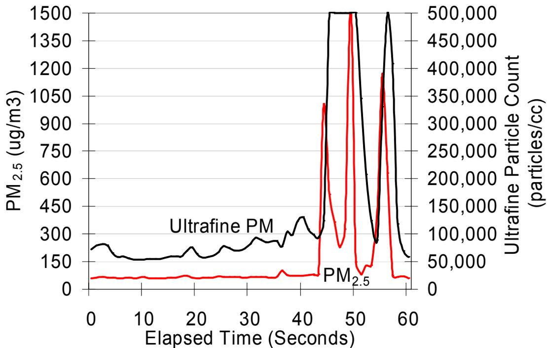
**Figure 48:** Simulation of school bus drop-off scenario on conventional bus shows large spikes in PM<sub>2.5</sub> as bus pulls up and then pulls away from the curb.
