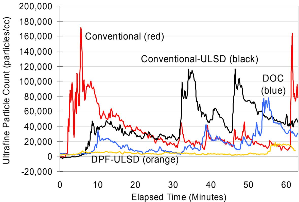
**Figure 21:** Comparison of ultrafine particles on the conventional, ULSD-only, DOC and DPF-equipped buses. The DPF-ULSD combination (flat orange line) is the only device that eliminates the in-cabin ultrafine particles. Ambient concentration has been subtracted.
