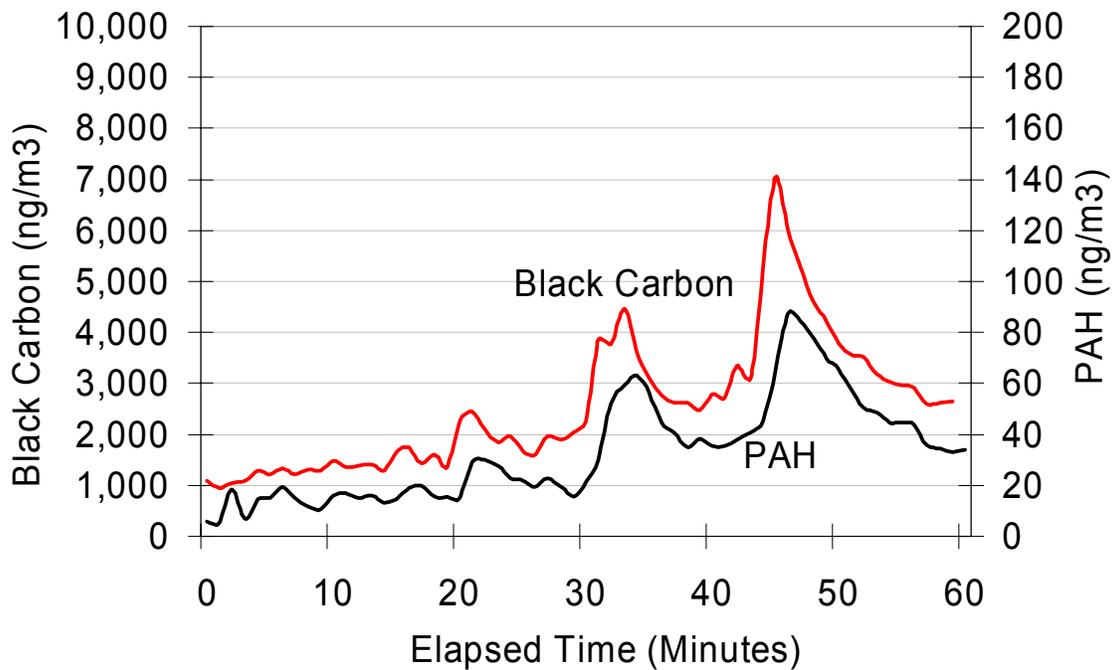
**Figure 40:** The Spiracle alone showed no apparent benefit in reducing black carbon and PAH levels.
