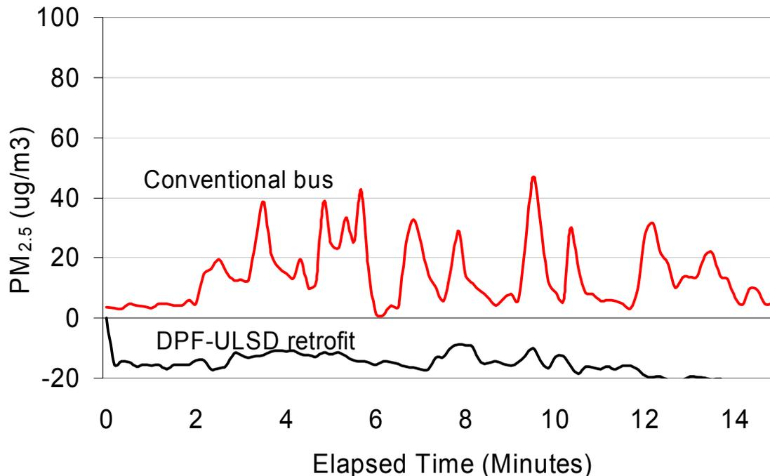
**Figure 53:** *PM<sub>2.5</sub> levels behind the school bus are strongly impacted by emissions from an unmodified conventional bus. In contrast, the bus retrofit with the DPF-ULSD shows little or no impact on the trailing car. This demonstrates the effectiveness of the DPF-ULSD combination in reducing ultrafine particulate matter in schoolyards and roadways and for queued buses leaving schoolyard and fleet lots. Ambient concentration has been subtracted.*
