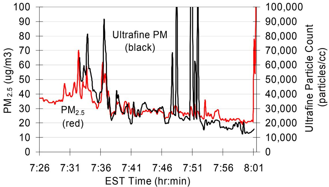
**Figure 51:** *PM<sub>2.5</sub> and ultrafine PM levels during morning school bus drop off at CT elementary school. Spikes in particulate matter occurred when buses left the school after dropping off children, leaving a cloud of diesel smoke in their wake.*
