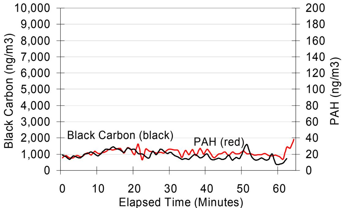
**Figure 41: PAH and black carbon self-pollution is reduced to ambient levels by the DPF in the ULSD-DPF-Spiracle combination. (Ann Arbor data.)**
