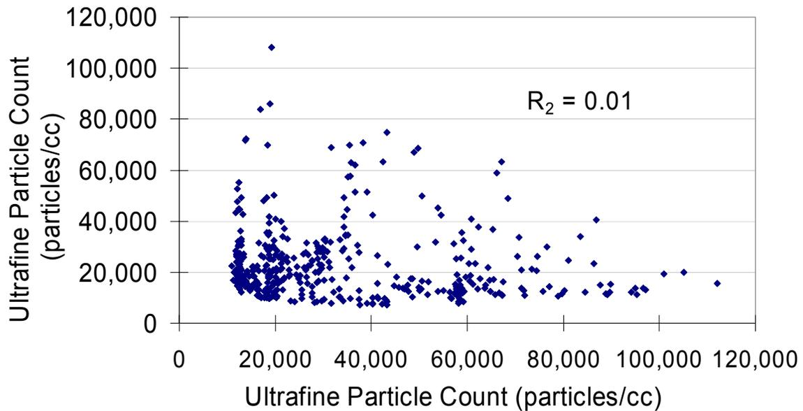
**Figure 13:** *Linear regression of ultrafine PM levels in bus with a 10 second lag (to compensate for time for emissions to penetrate bus) with ultrafine PM in lead car. Suggests no predictable relationship between roadway exhaust and cabin exhaust.*
