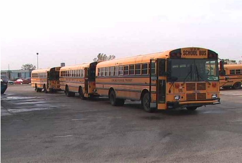
**Figure 43: Bus queue in Chicago.** Here, three transit-style buses were lined up in a common safety protocol allowing no walking space between buses (so that children cannot walk between buses.) This puts the tailpipe of one bus near the door of the one behind it and accounts for the dramatic increases in particulate matter levels when the doors are open and the buses at idle.
