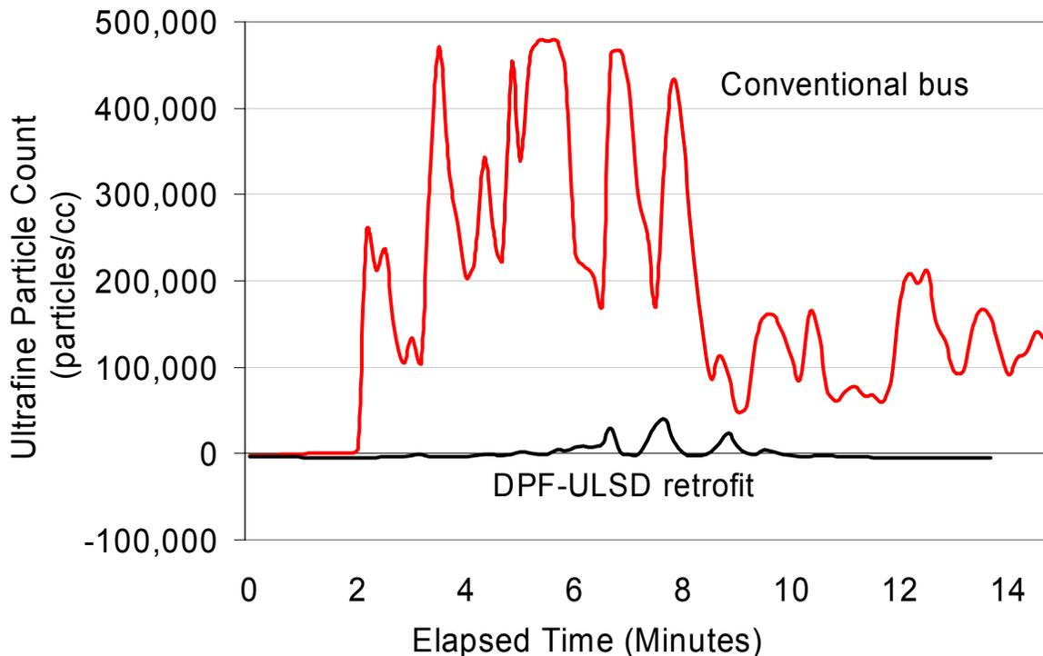
**Figure 52:** *Ultrafine particulate matter behind the school bus are strongly impacted by emissions from an unmodified conventional bus. In contrast, the bus retrofit with the DPF-ULSD shows little or no impact on the trailing car. This demonstrates the effectiveness of the DPF-ULSD combination in reducing ultrafine particulate matter in*
