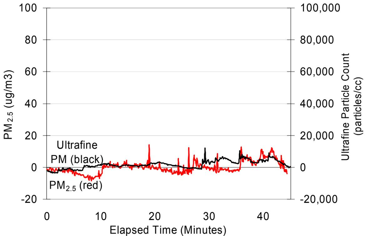
**Figure 30: Fine particulate matter ( $PM_{2.5}$ ) levels on retrofit DeKalb GA bus #1450 following retrofit and addition of a simple extension of the road draft tube). In this run, the extension tube effectively redirected the crankcase emissions so they did not enter the bus. However two other runs with the extension tube exhibited significant  $PM_{2.5}$  influx (Table 7). Ambient concentrations have been subtracted.**
