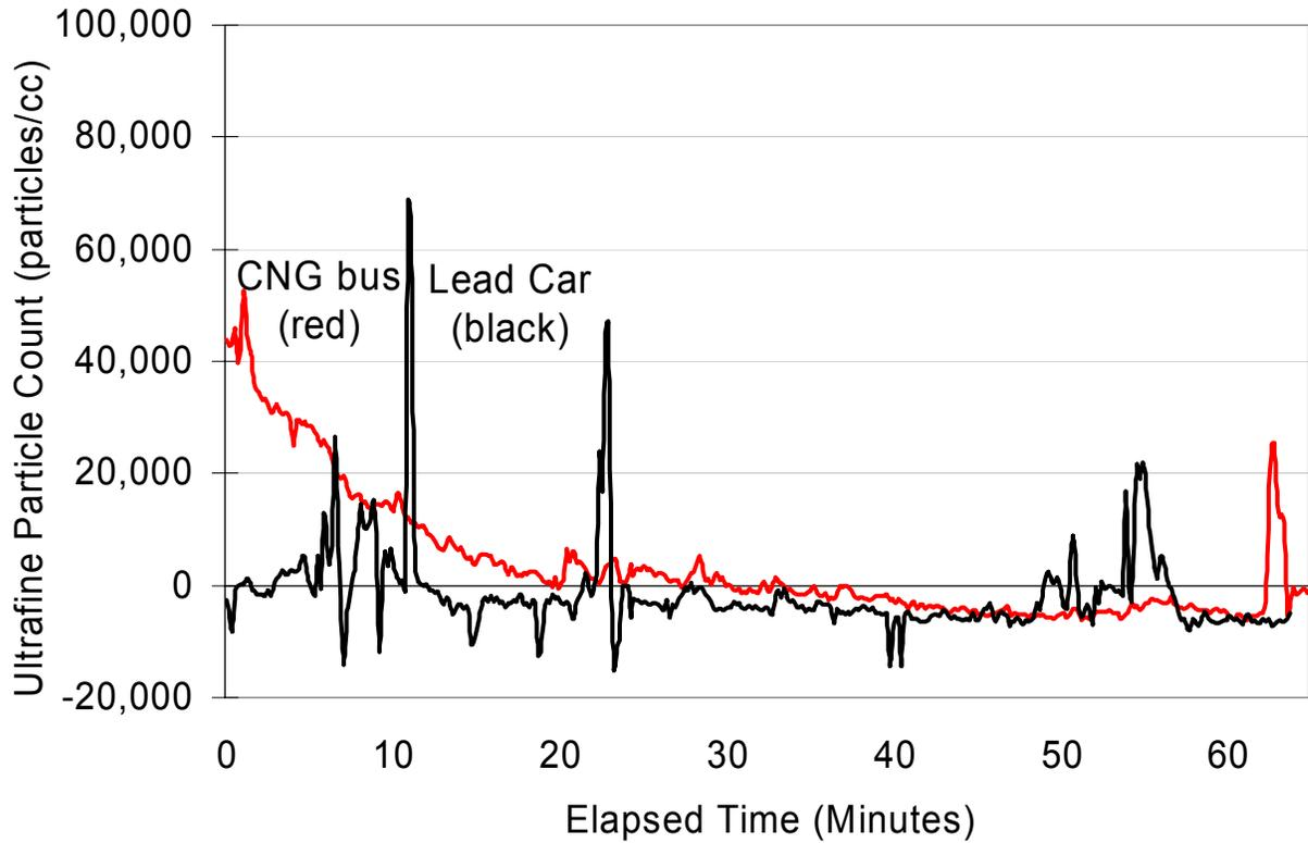
***Figure 22: Ultrafine PM in Ann Arbor transit-style compressed natural gas (CNG) bus #24 compared to lead car. Ultrafine PM was detected in the cabin of the CNG bus from the bus and traced to its tailpipe which was on the driver's side, farthest from the cab. The initial particle concentration build up on the graph occurred during idling. Ambient concentration has been subtracted.***
