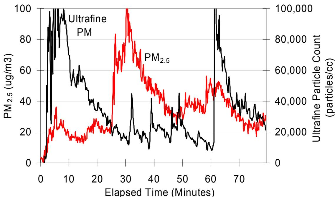
**Figure 1: Conventional buses tested showed significant PM<sub>2.5</sub>, ultrafine particle, black cabin and PAH self-pollution. (Ambient concentrations have been subtracted.)**
