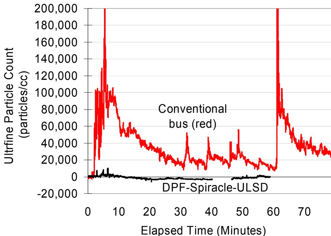
**Figure 32:** Comparison of ultrafine particle levels on a conventional bus and bus equipped with the DPF –ULSD – Spiracle combination. Ambient concentrations have been subtracted which may result in a false negative net ultrafine count. Ambient concentration has been subtracted.
