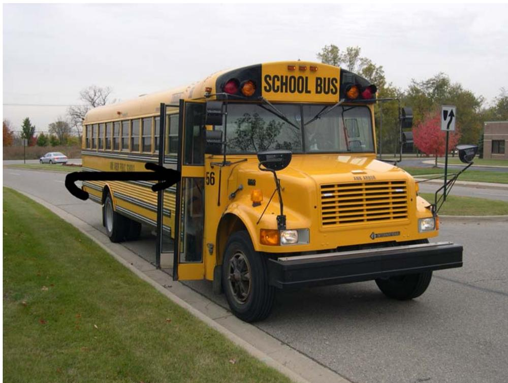
**Figure 14:** Schematic of bus tailpipe plume entrained from rear toward bus door..
