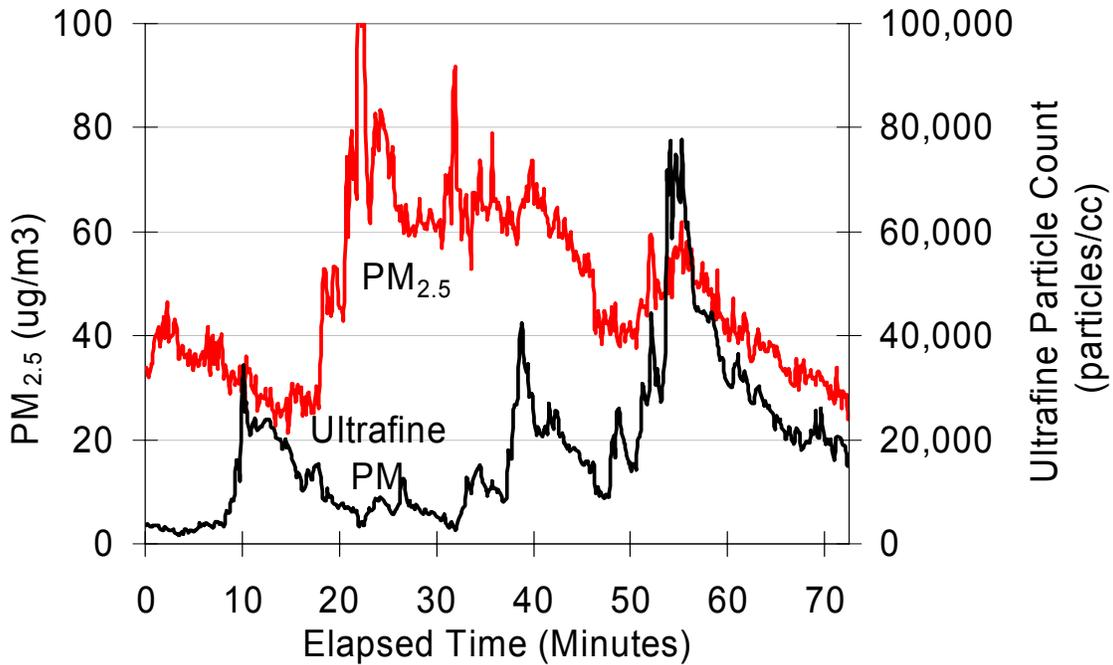
**Figure 56:** *PM<sub>2.5</sub> and ultrafine particle concentrations remain substantially elevated on bus retrofit with DOC. Black carbon and PPAH were also elevated. Ambient concentrations have been subtracted. (Ann Arbor data.)*
