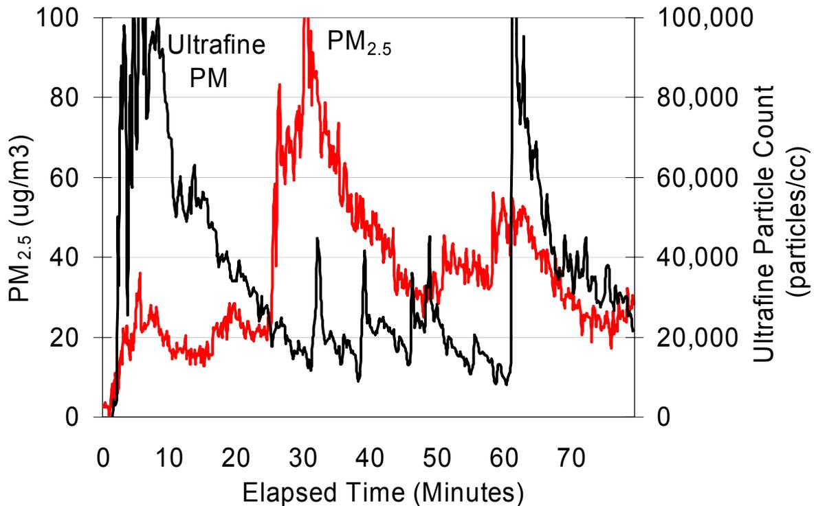
**Figure 55: High PM<sub>2.5</sub> and ultrafine particle concentrations in a conventional bus indicate significant cabin self-pollution. Black carbon and PPAH were elevated as well (see previous section.) Ambient concentrations have been subtracted. (Ann Arbor data.)**
