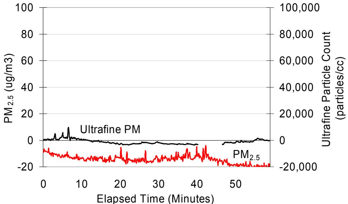
**Figure 59:** *PM<sub>2.5</sub> and ultrafine particle concentrations on bus #56 retrofit with DPF-ULSD-Spiracle shows reduction in all cabin particulate matter parameters measured approximately to ambient or slightly below. Ambient concentrations have been subtracted. (Ann Arbor data.)*
