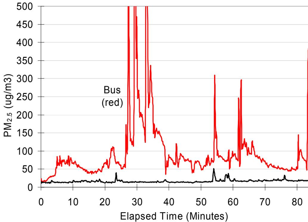
**Figure 11:** *PM<sub>2.5</sub> in the bus cabin is not from the roadway but instead result from bus self pollution-- as indicated by the low concentrations in the lead car relative to the bus.*
