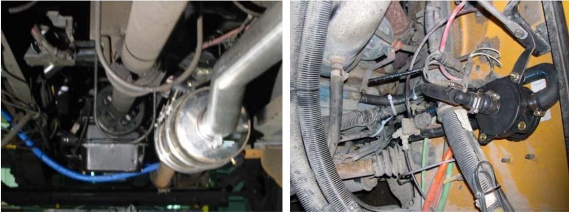
**Figure 29: Experiments to mitigate smoke from road draft tube. (a) Left: Simple blue plastic extension of road draft tube (Atlanta). (b) Right: Enviroguard “blow-by” filter (black) attached to road draft tube (Ann Arbor.)**
