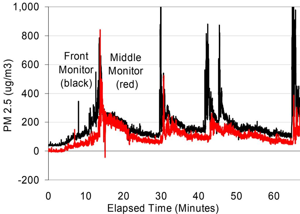
**Figure 10:** Comparison of  $PM_{2.5}$  concentrations between front and middle of bus in Chicago. Note the parallel signatures with levels exceeding  $1,000 \text{ ug/m}^3$  in the front of the bus. Levels in the middle of the bus are lower and slightly lagging. This supports
