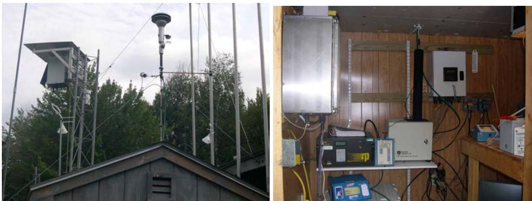
**Figure 5: Camp Dodge Monitoring site where Dust Traks were co-located with TEOM, IMPROVE and Harvard Impactors for 13 days.**
