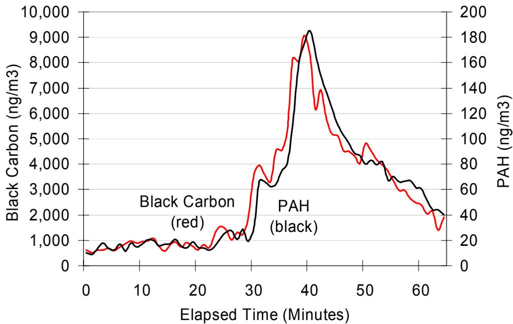
**Figure 39:** PAH and black carbon levels are unimproved with the DOC-Spiracle combination in Ann Arbor, MI.
