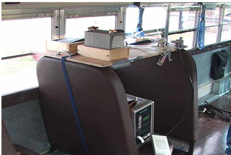
**Figure 4: Bus instrumentation in Chicago. Dust Trak and Aethalometer on bus #662. The Dust Trak was operated with a Nafion Tube dryer-pump assembly. Not shown: PTrak ultrafine particle counter and PAS 2000 (PAH.)**
