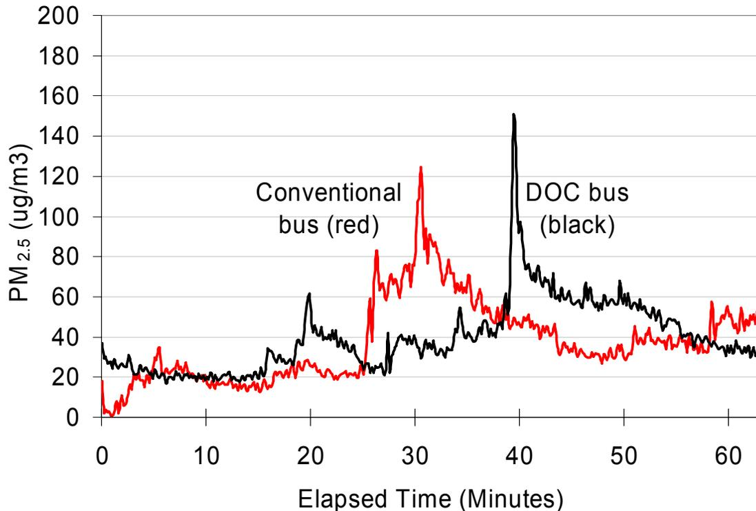
**Figure 34:** *PM<sub>2.5</sub> on bus equipped with a DOC compared to conventional bus in Ann Arbor, MI. Cabin PM<sub>2.5</sub> remains elevated with DOC. Ambient concentration has been subtracted.*
