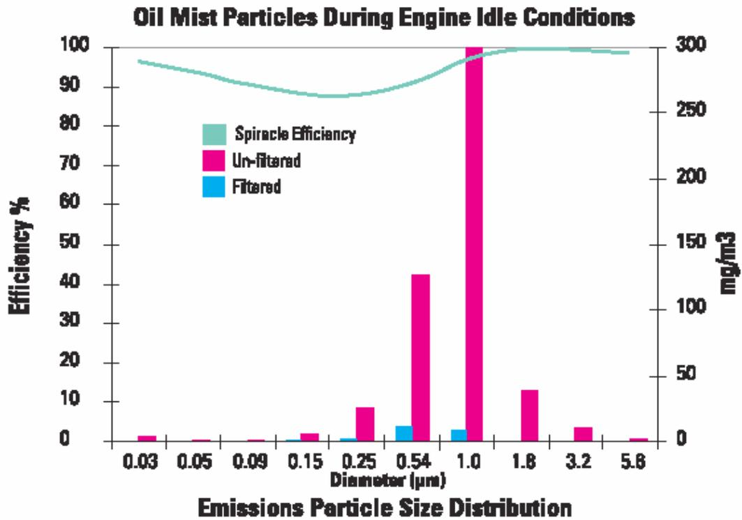
Figure 27: Size distribution of particles from crankcase blow-by. (Source: Donaldson.)<sup>65</sup>
