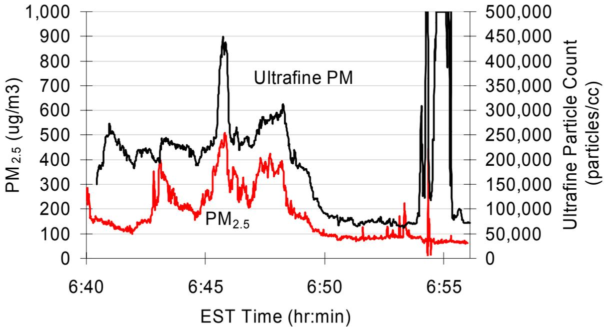
**Figure 47:** Particulate matter levels rise to high levels in fleet bus lot in Atlanta as buses warm up prior to morning bus routes. The idling emissions strongly affected the cabin air of all buses in lot and the smoke diffused into the adjacent residential area.
