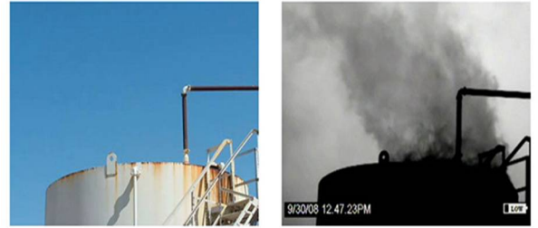
Above: Advanced imaging shows methane leaks from existing gas infrastructure, which was largely unaddressed in EPA's rule.
