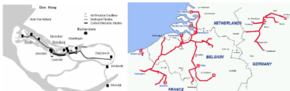
Figure 10: Existing hydrogen pipelines operated by Air Products (left) and Air Liquide (right) (DNV, 2017)
