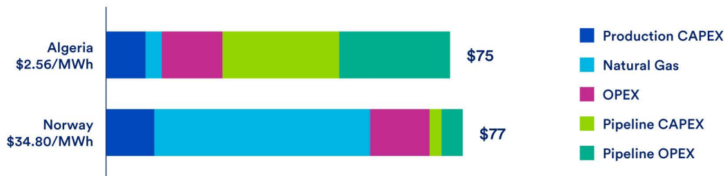
Figure 13a: Cheapest Hydrogen Production Transported to Rotterdam via Pipeline ($/MWh H 2 ) 1 Million Tonnes Per Year H 2 Supply Chain (2040)
