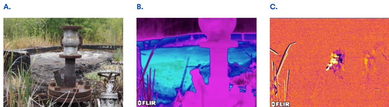
Figure 3: Difference Between Normal and Enhanced Operating Modes for an OGI Camera
